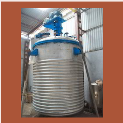
Limpet Coil Reactor
