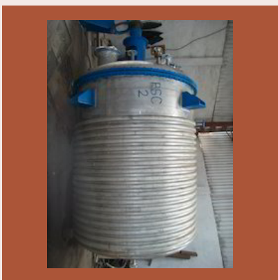
SS Coil Reactor
