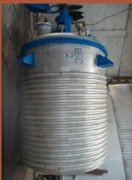
SS Coil Reactor
