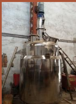
GMP Jacketed Reactor
